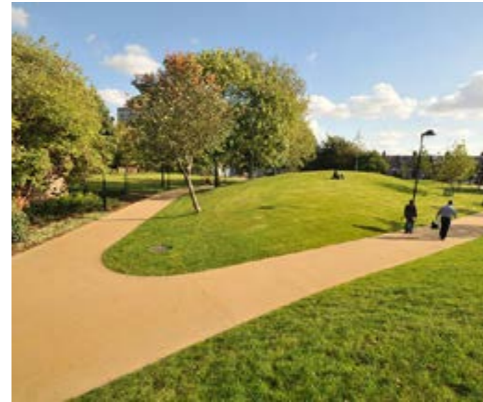
Pathway / Resin bound gravel appropriate to routes through green park spaces.
