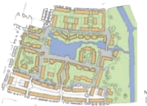
Ecolonia's layout is centred on a reed-fringed pond, with buildings orientated to maximise solar gain
