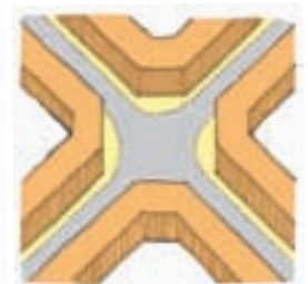
Rotating the building line to create a square on the diagonal as in Barcelona
