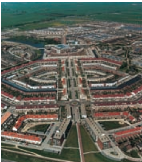
Sheets, blocks and buildings are orientated for solar gain (Photographer: Jan van Ijken)
