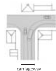
Tighter kerb radii can be used with a wider carriageway. The refuse vehicle turning requirement is still accommodated, yet vehicles do not dominate
