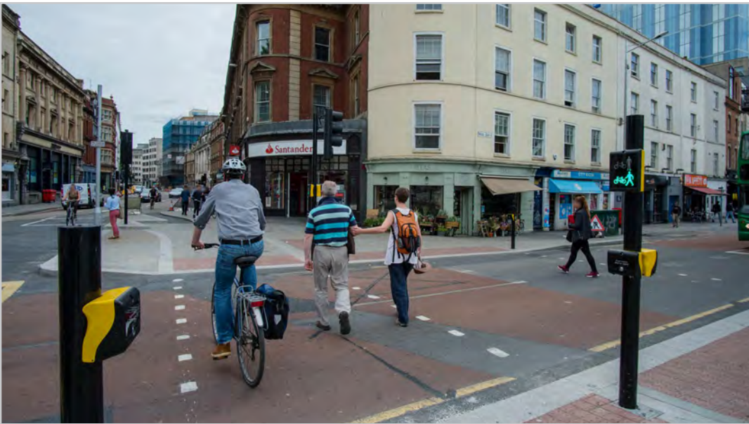
Signalised crossing Signal-controlled crossings comprising either a Pelican/ Puffin for pedestrians or a Toucan which can be shared between pedestrians and cyclists.
