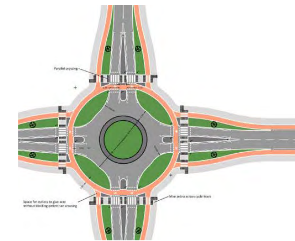
Figure 10.37: Roundabout with one way cycle tracks and parallel crossings
