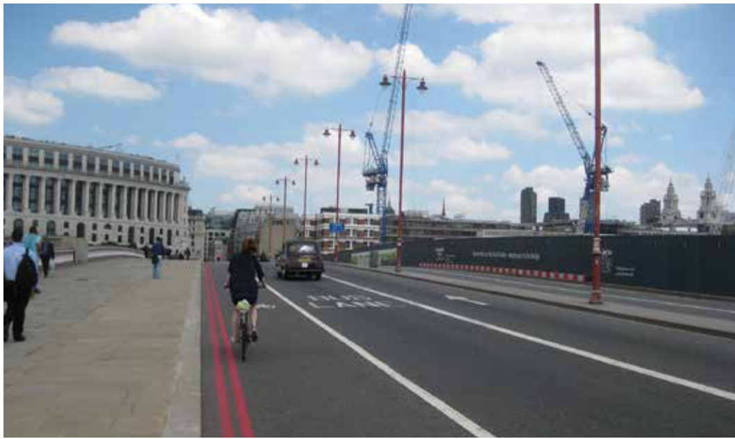
Mandatory cycle lane Area of the carriageway reserved for the use of cycles, marked with a solid white line.
